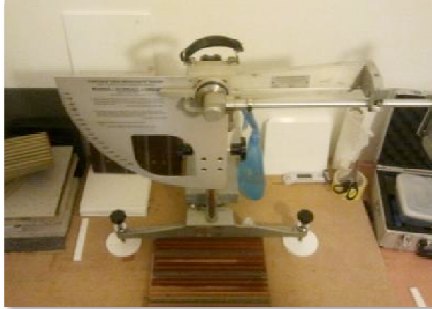
Image 1. Pendulum tester in-situ
