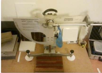
Image 1. Pendulum tester in-situ
